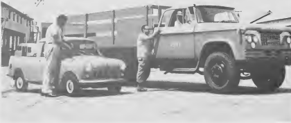
THE TOP OF the diminutive pick-up truck at left barely reaches the platform level of a big LAGO platform truck. The little fellow is an Austin Seven from England and is one of four being tested by LAGO. It has a ten cu in. engine and a capacity of 500 lbs. The big Dodge has a six-ton capacity.
